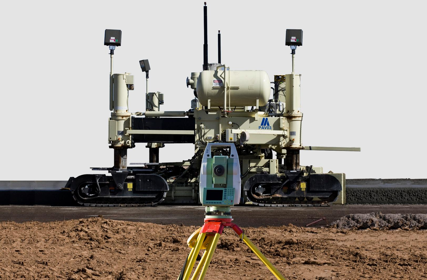
The NoLine: Stringless Preparation Kit can be included as an option on all G&Z Pavers and Support Equipment. NoLine is comprised of a software upgrade and a hardware kit. The NoLine Software Upgrade integrates the use of stringless technology directly into the machine's CANBus network. The NoLine Hardware Kit provides telescopic masts for the total station prisms (only necessary on pavers) and battery backup. NoLine makes paving stringless easy through reliable, proven and integrated software.
